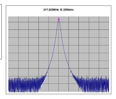
10/05/2007 Centre Frequency: 217.02500MHz Resolution Bandwidth: 30kHz Span: 2MHz Video Bandwidth: 100kHz Sweep Time: 50 ms Attenuation: 30 dB Reference Level: 46.16 dBm Marker Amplitude: 29.83 dBm Power: .9616 Watts
