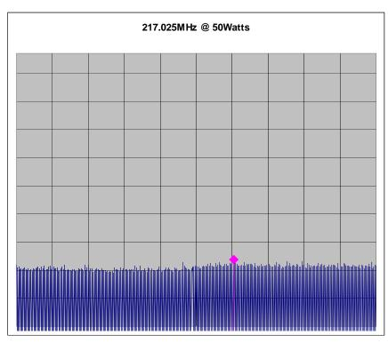
10/05/2007 12:13 Centre Frequency: 2G Resolution Bandwidth: 10KHz Span: 4GHz Video Bandwidth: 30kHz Sweep Time: 100sec Attenuation: 20 Reference Level: 30.16 Marker Amplitude: -73.67dBC
