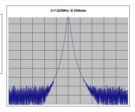
9/05/2007 Centre Frequency: 217.02500 MHz Resolution Bandwidth: 30kHz Span: 2MHz Video Bandwidth: 100kHz Sweep Time: 50 ms Attenuation: 30 dB Reference Level: 46.16 dBm
