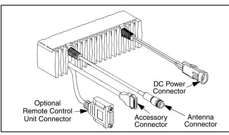
**DC** Power Connector – Connection point for the nominal 12-volt, negative ground power source.
