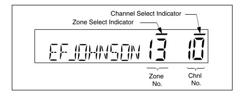
The selected zone and channel is changed by the front panel Select switch as follows:
