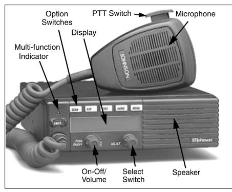
**On-Off/Volume** – Pressing this control turns power on and off, and rotating it sets the volume level.
