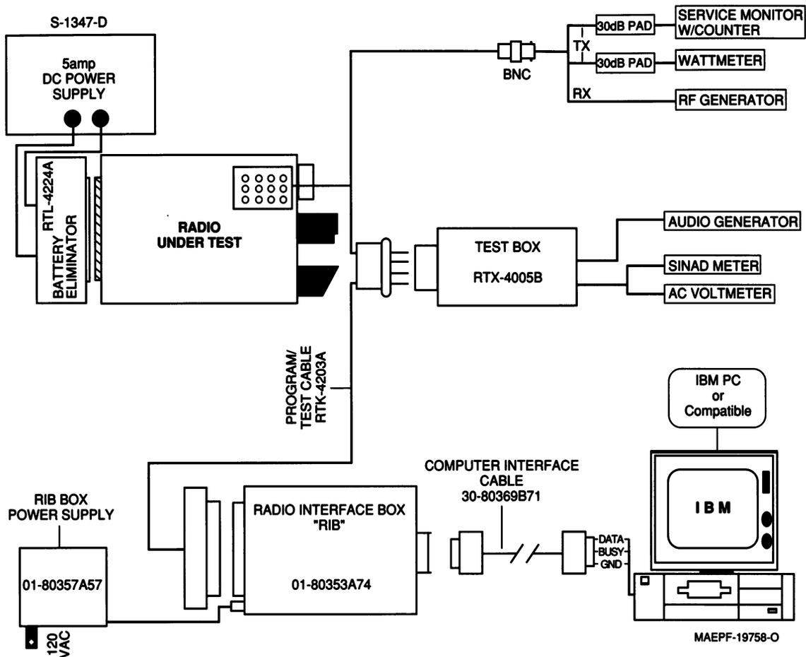
Figure 5. Troubleshooting, Programming, and Test Equipment Setup Detail
