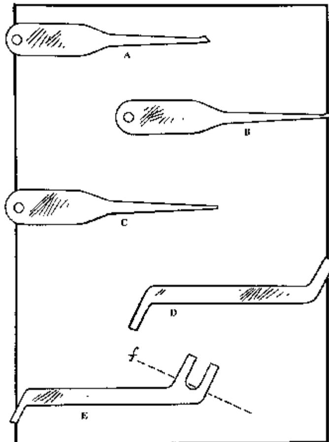
**Figure 3. A: a diamond pick; B: a small diamond pick; C: a tubular cylinder lock pick; D: a tension wrench, used with the diamond picks; E: a tension wrench intended for double-wafer cylinder locks and tubular cylinder locks.**
