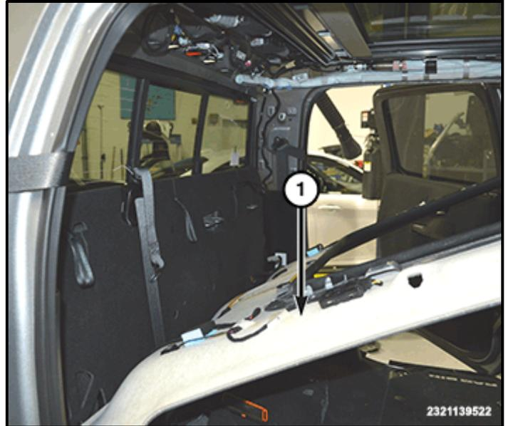
4. Insert a 4 mm hex tool into the screw (1) and rotate the motor as necessary to move the sunshade about 100 mm (4 inch) forward from the full rear position.
