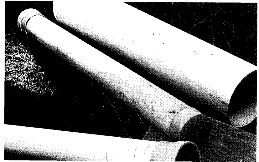
Cache tubes showing both permanent and access ends.
