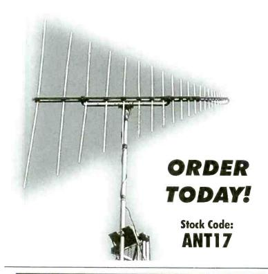
The log-periodic dipole array (LPDA) is respected for its wide bandwidth, constant impedance, and high gain. Measuring 4'10" boom length, the Create CLP-5130-2N (our catalog no. ANT-17) offers 100-1300 MHz bandwidth for transmitting and receiving, with an average forward gain of 11-13 dBi. Ruggedly constructed of solid aluminum for lightweight durability. Fitted with an N connector for low-loss coax.
