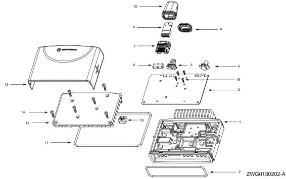
Figure 3-10 Radio Assembly - 25W Models
