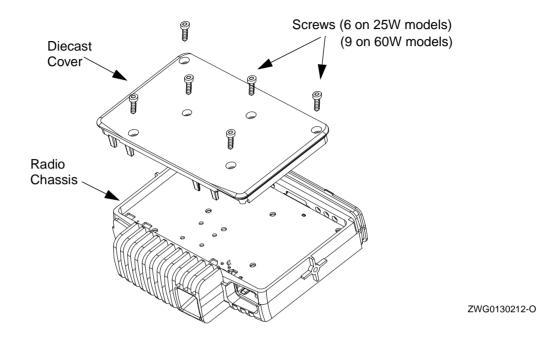
Figure 3-4 Diecast Cover Removal.
