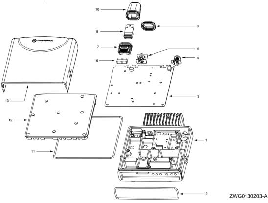
Figure 3-11 Radio Assembly 60W Models
