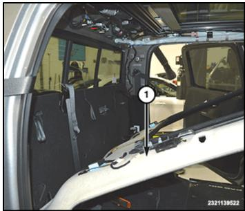
4. Insert a 4 mm hex tool into the screw (1) and rotate the motor as necessary to move the sunshade about 100 mm (4 inch) forward from the full rear position.
