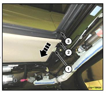
10. Pull the sunshade (1) out far enough to access the spacer (2). Remove the spacer by hand.
