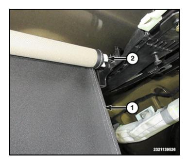
7. Align the tension bar end (1) with the sunshade fabric.
