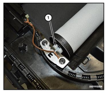
12. Grasp the sunshade on the right side of the vehicle and slide it to the left, then remove the end (1) from the pivot bracket (2).
