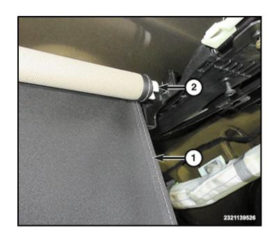
11. This graphics shows the spacer (1) from the top-side, push on the spacer till it snaps-off the sunshade shaft.
