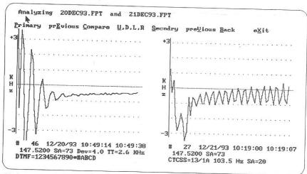
This is an example of the TxID Software Comparison feature. The fingerPrints shown were actually captured by the TxID-1.
